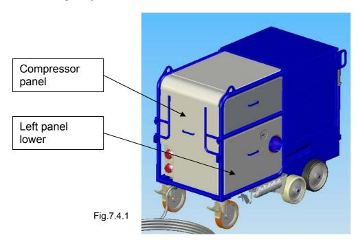
The V-belt drive is located behind the Compressor panel. The V-belt tension device is located behind the Left lower panel.
