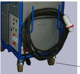
The dustcollector is equipped with a cable support. Wrap the supply cable over it in order to avoid damaging during transport.
